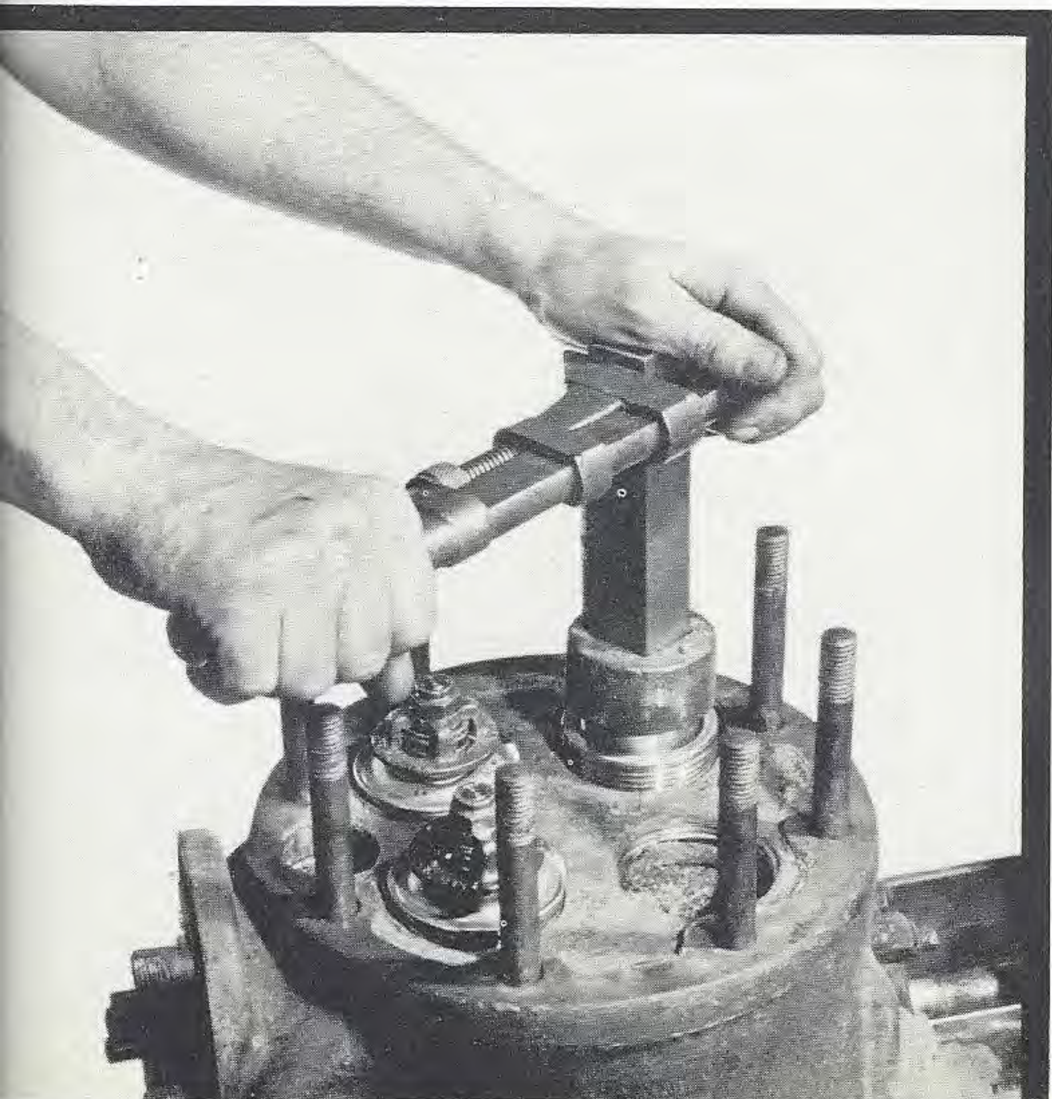
Fig. 10 — The seat wrench securely grips the webs.
