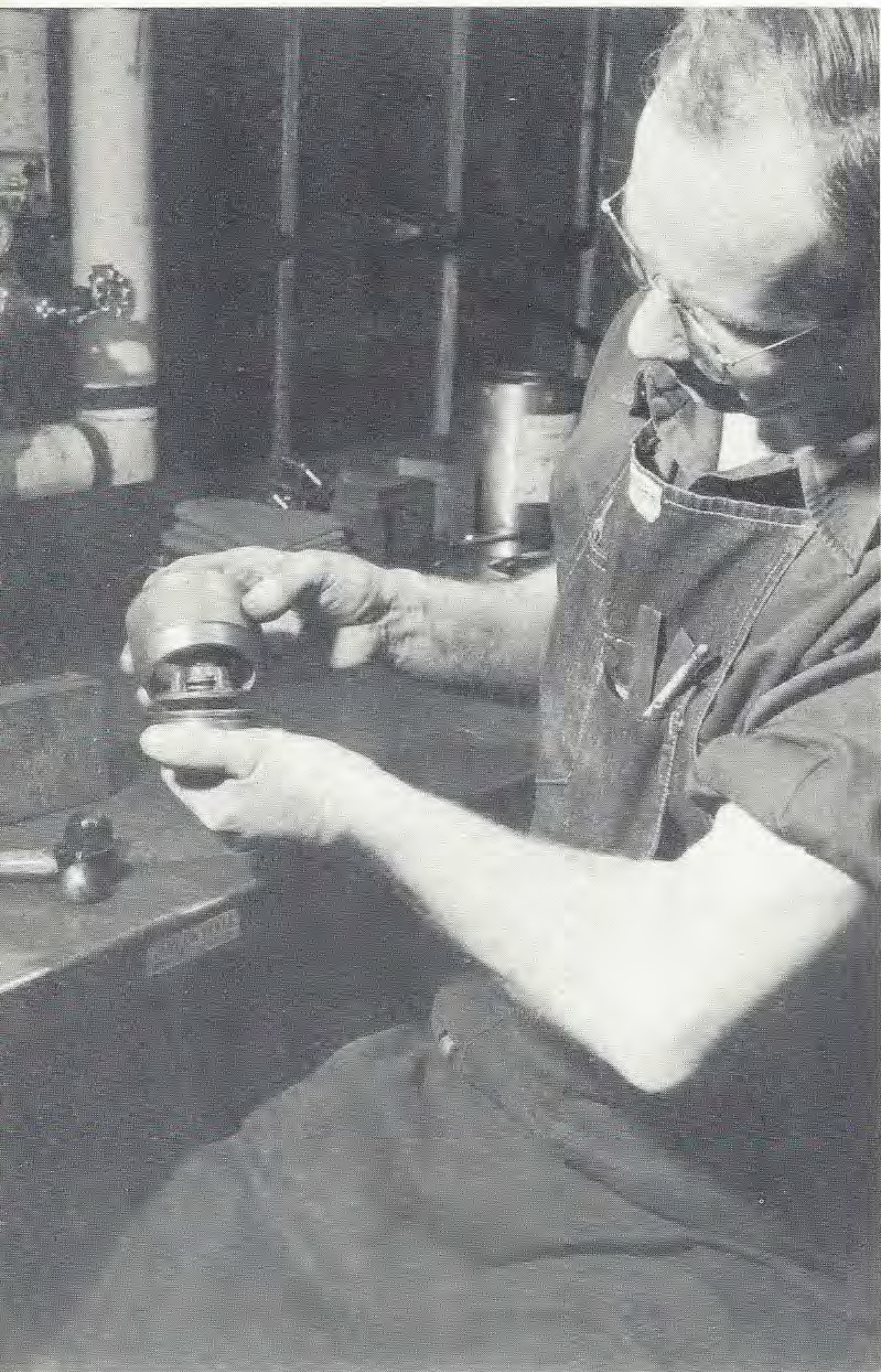
Fig. 6 — Accuracy of fit of pressing block should be checked.
