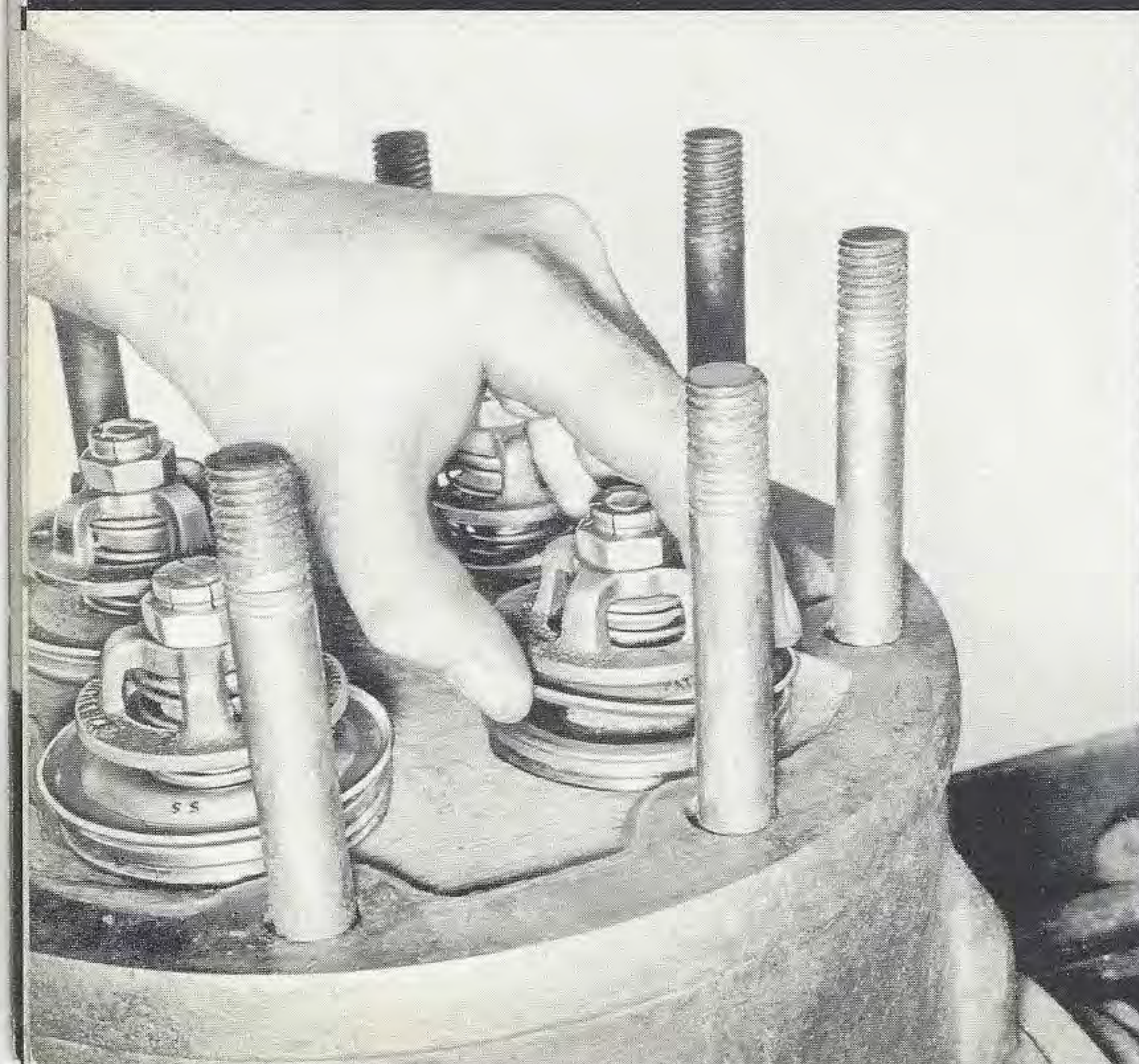
Fig. 8 — Don't fail to “try” the valves before closing the pump.
