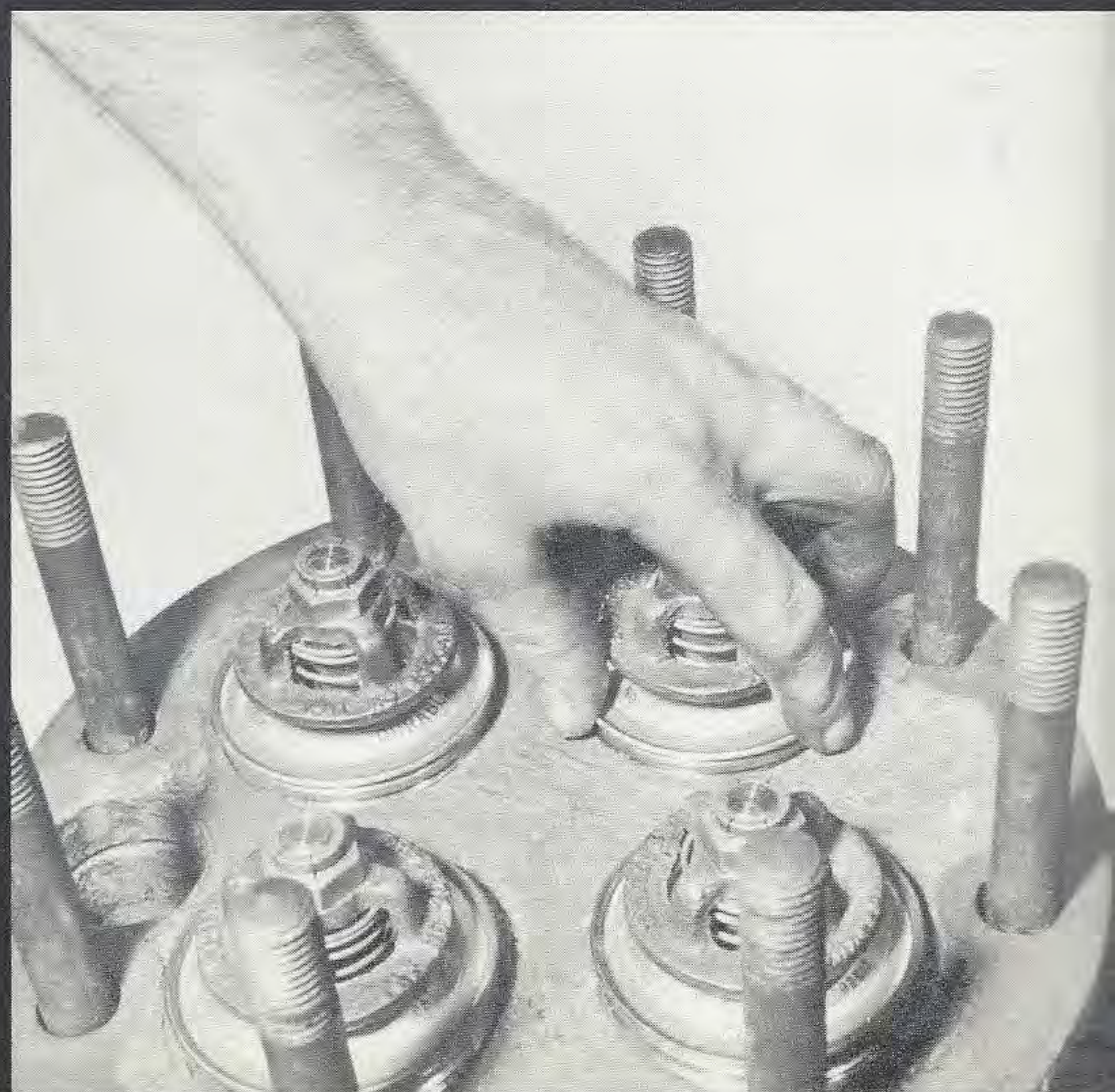
Fig. 9 — The final check of rotating the valve.
