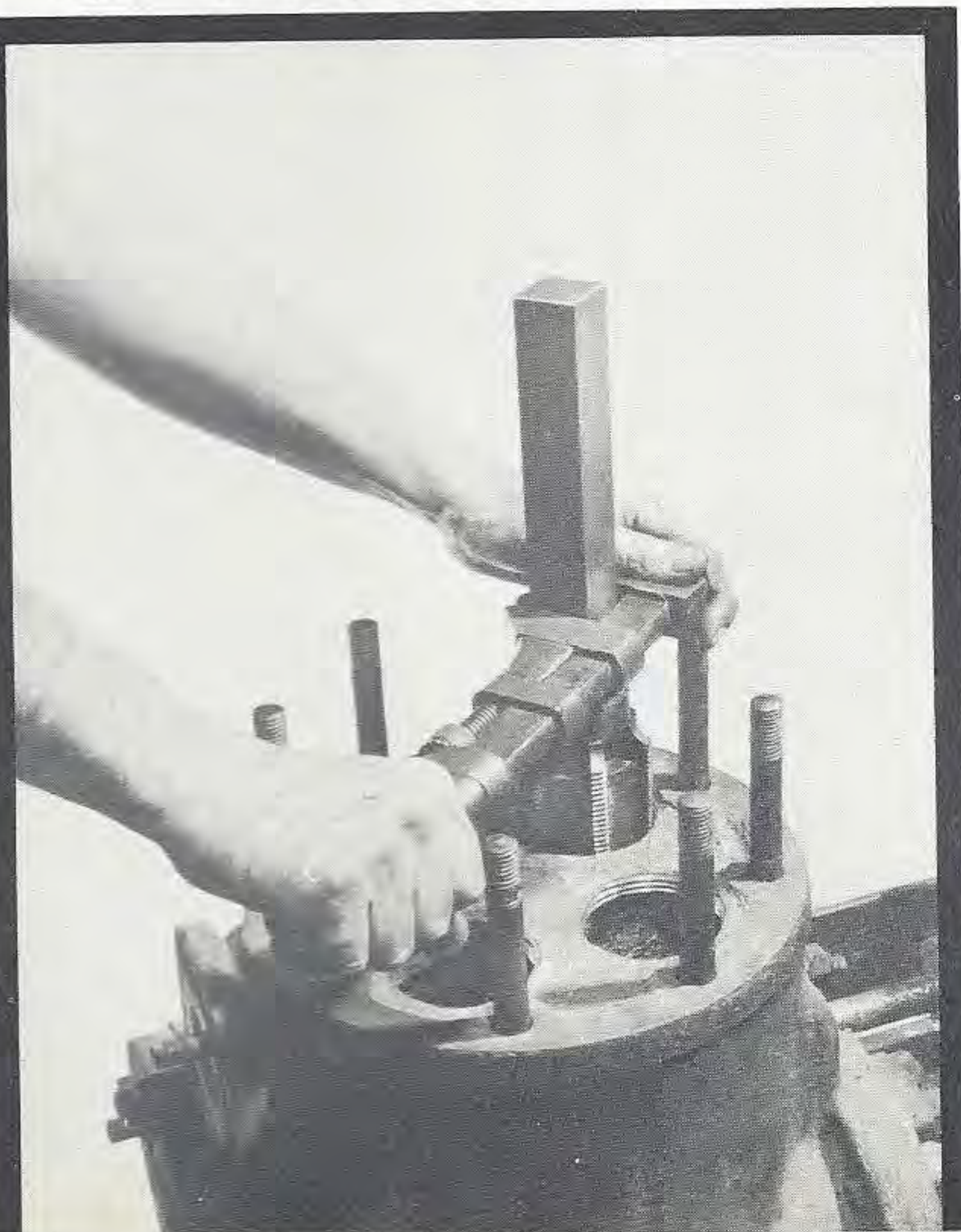
Fig. 5 — Using tap to insure clean threads.
