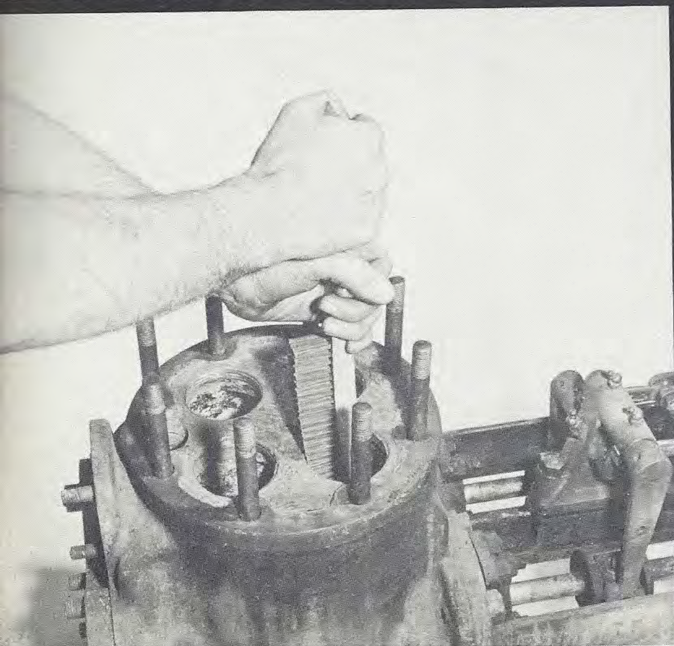
Fig. 4 — Wire brushing to remove corrosion.
