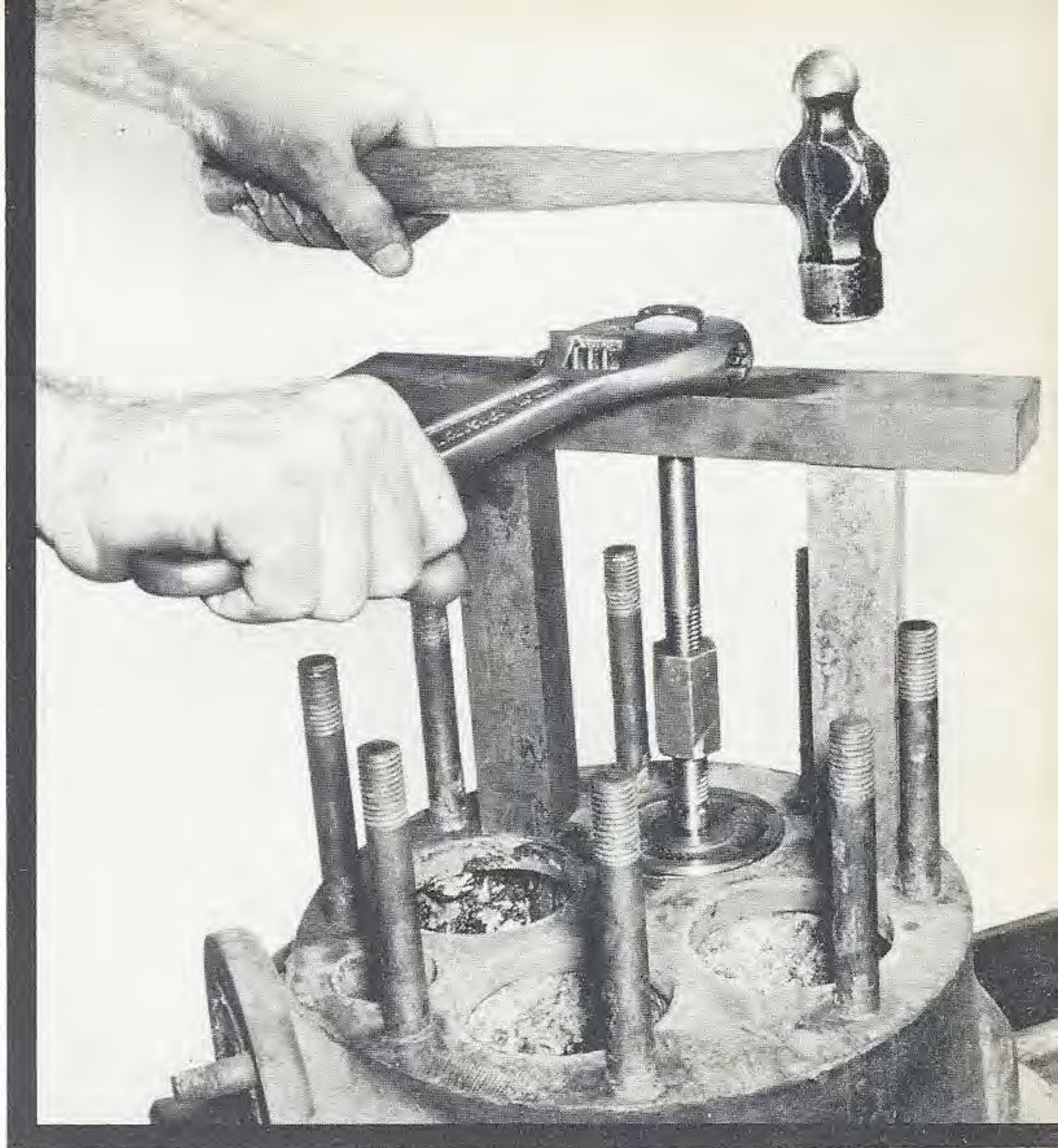
Fig. 13 — Using the strong-back to grip the stud.
