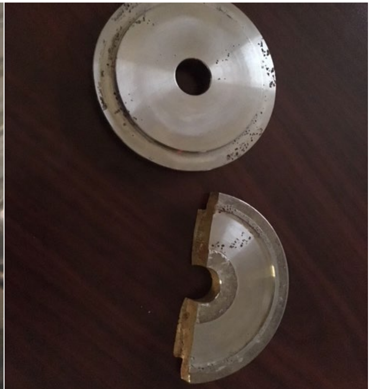
Valve disc showing pitting caused by cavitation.
