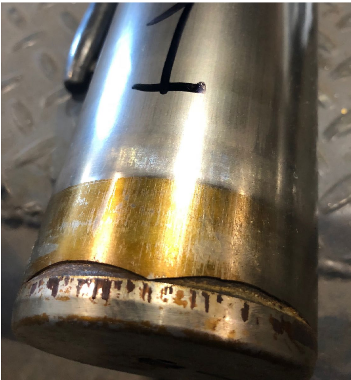
Spray metal plunger showing damage caused by severe cavitation.
