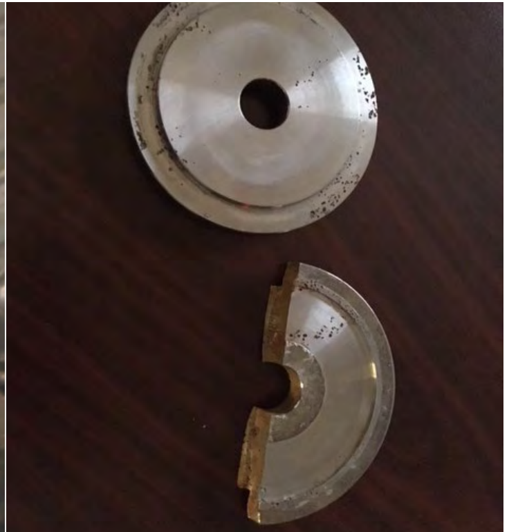
Valve disc showing pitting caused by cavitation.
